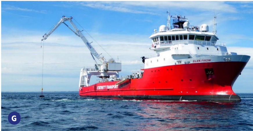
E MV Elektron – Cable repair vessel loading replacement cable in Vlissingen F 1 of 4 CTVs utilised on the repair project to cover 24/7 ops on OSS, TPs, CLV, DSV G MV Elektron and its back deck setup
