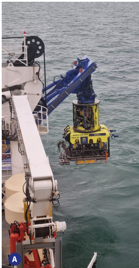
A ROV XLX49 Deployment B ROV XLX49 on deck C Deployment of CFE tool D Sub Bottom Imager 'Kraken' tool underneath ROV E ROV XLX49 ready for launch
