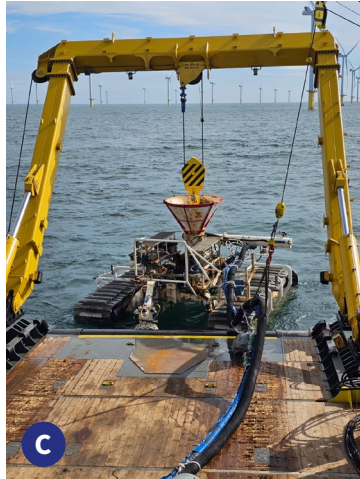
A Cable lay vessel CURO B Quadrant deployment for second end pull-in C Launch mechanical trencher D Fist end cable recovery to deck E Cable loading with powered quadrant
