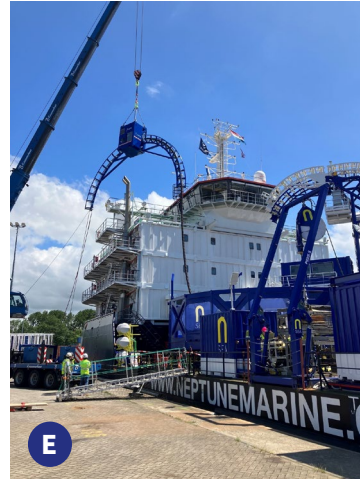
A Cable lay vessel CURO B Quadrant deployment for second end pull-in C Launch mechanical trencher D Fist end cable recovery to deck E Cable loading with powered quadrant
