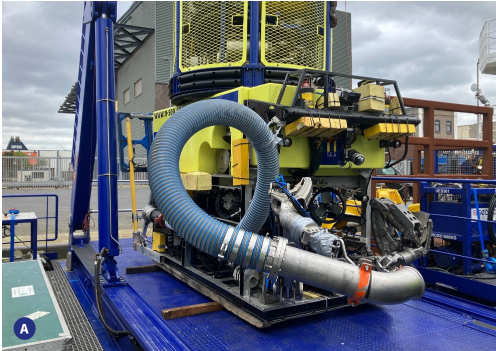
A WROV TXL17 with subsea dredging hose B WROV with installed manipulators
